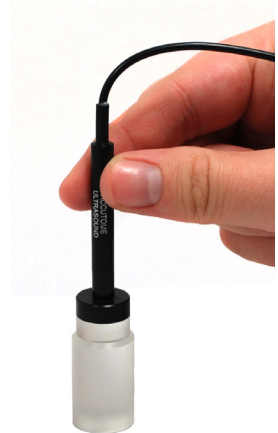
Figure 9.6 - Using the A-Scan Test Block
